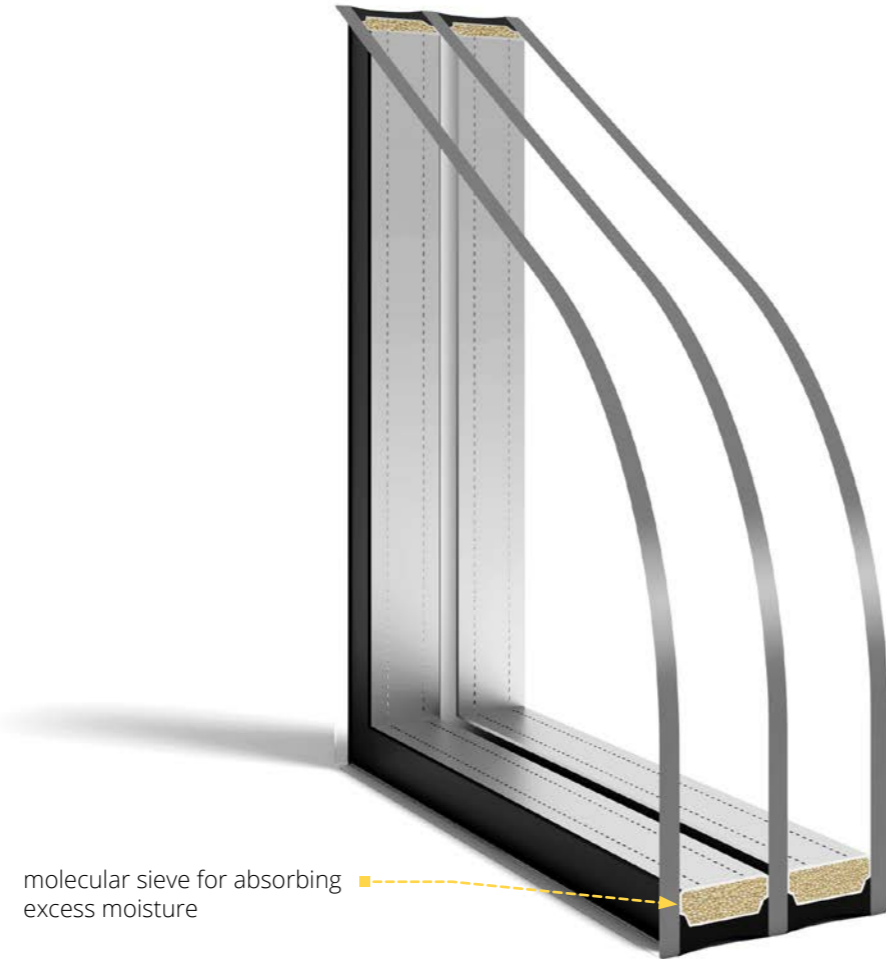
3-pane (2-chamber) 48 mm units with glass-pane spacer made of galvanised steel.
